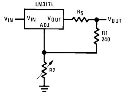
FIGURE 2. Regulator with Line Resistance in Output Lead
